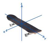
We then consider an orthonormal frame  $\vec{v}_1, \vec{v}_2, \vec{v}_3$  which is locked onto the skateboard and based at its center of mass.
